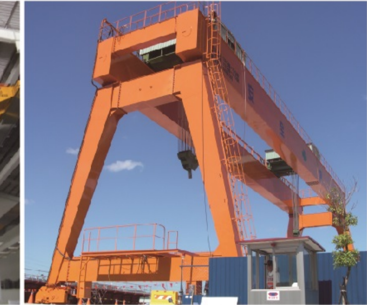
2010 Airport Metro Line 260 Tons Gantry Crane Project
